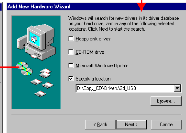
Dialog 3: Use the button <Browse> to select the following directory: "D:\COPY_CD\DRIVERS\2D_USB" (Given D:\ is the drive letter of your CD-ROM drive)
